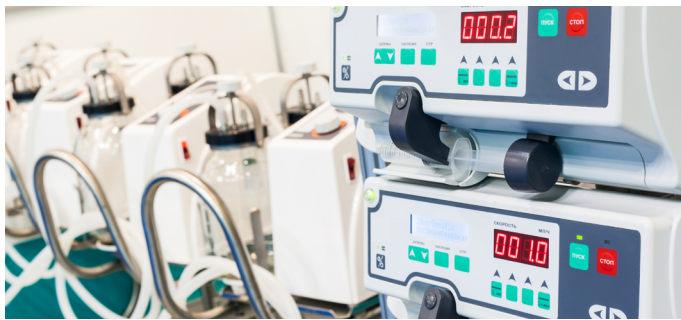
MONITORING THE FLOW RATE AND/OR POTENTIAL OCCLUSION DURING INFUSIONS IS AN APPLICATION FIELD FOR LOW RANGE COMPRESSION LOAD SENSORS
