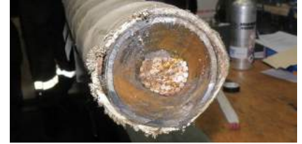
Sample of the 50 year old PILC oil paper cable.
